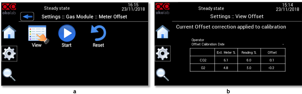
Figure 37. View Sensor calibration status
