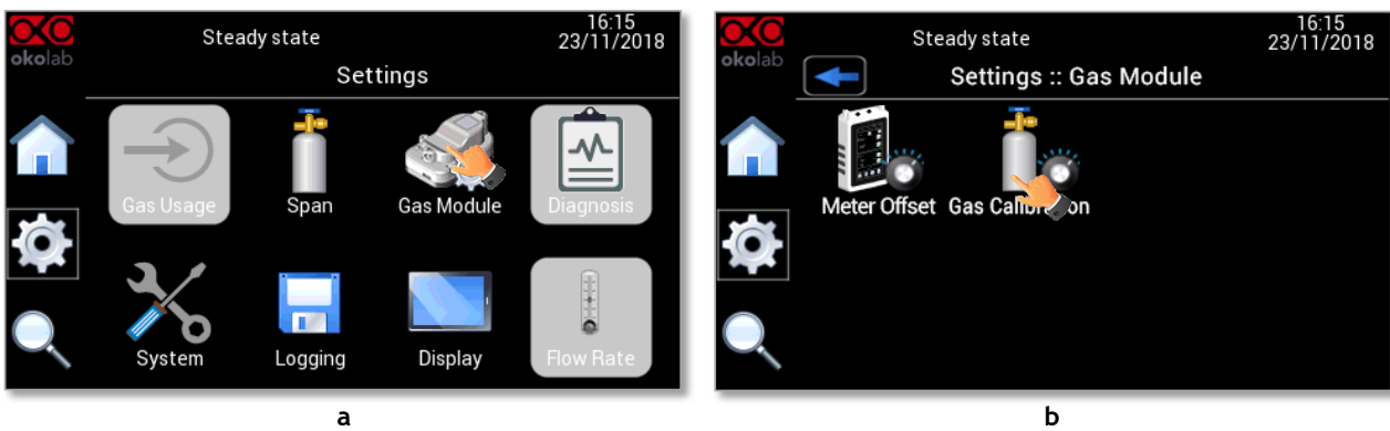
Figure 56 How to enter the Gas Calibration page
