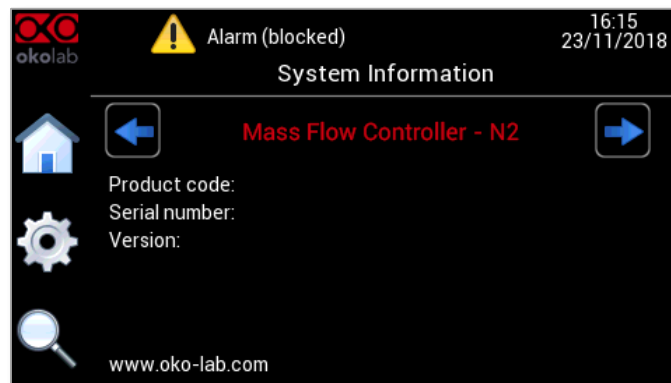
Figure 142. Message for mass flow controller improper installation
