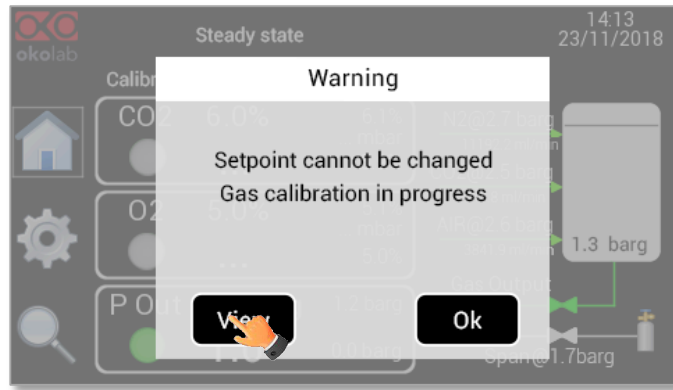
Figure 61 Warning appearing during the calibration procedure
